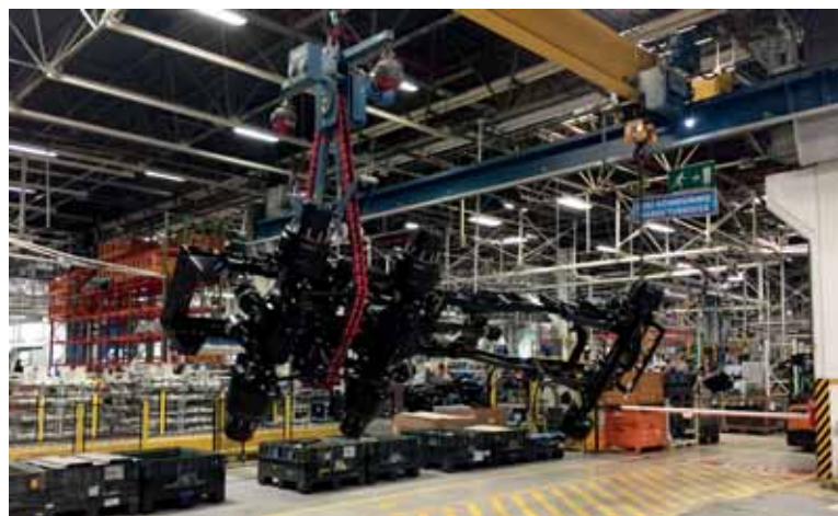
A truck chassis is flipped and rotated before it sits back down on a production line and is married to the cab
